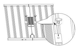
2. UNFOLD THE FIXTURE TRACK (FIG.A) AND PLACE IT ON A STURDY AND FLAT SURFACE WITH THE DIODE ARRAY FACING DOWNWARD.
